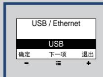
步骤 3 ▶ 选择“Ethernet”端口开启。按钮操作的顺序为：FEED -> PAUSE -> FEED
